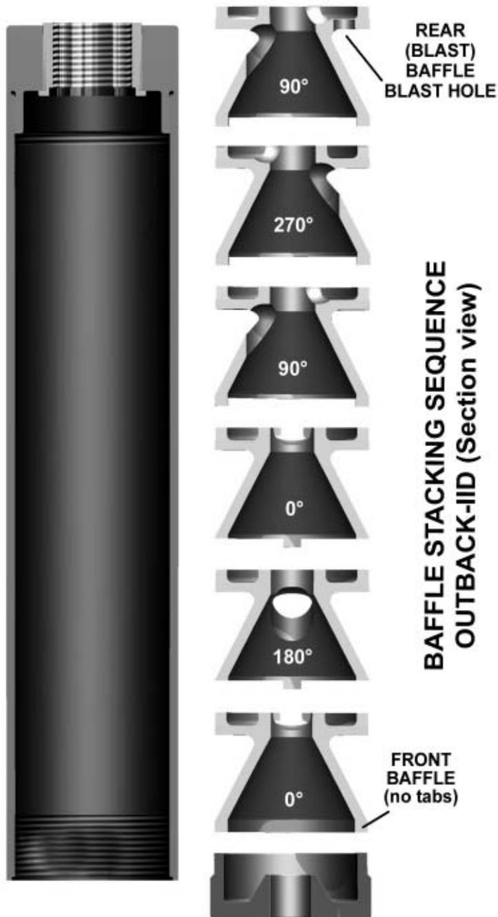
The simplest method of reassembly is to stack the baffles in the proper sequence and orientation on a 1/4 inch diameter rod or dowel approximately 6 inches long. Please refer to the drawing on page 7.
