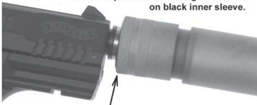
Silver band on black sleeve no longer visible. Suppresser is locked on mount and safe to shoot.
